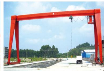
MH Gantry Crane With Electric Hoist
